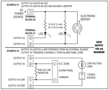
Figure 9. Using Solid State Outputs
